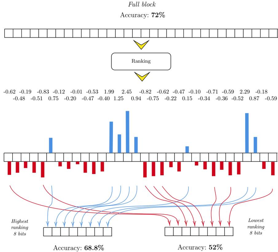
**Fig. 5.** The Training Process of PD-ML-distinguishers. Rank values are as per Table 1. Plotted bars are approximation of the values (due to graphical constraints).
