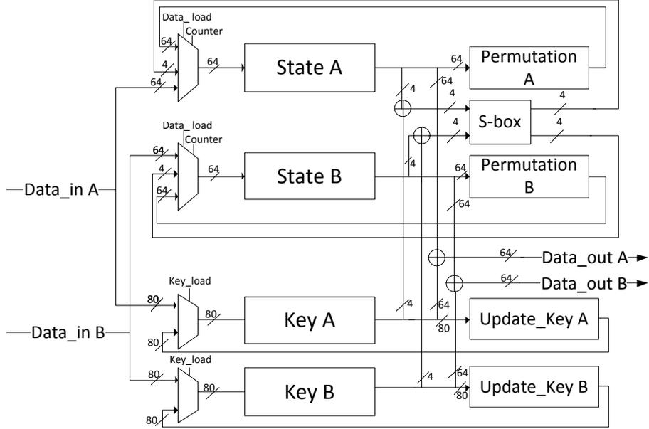
Fig. 4. Hardware architectures of the 2-shares Present Cipher.
