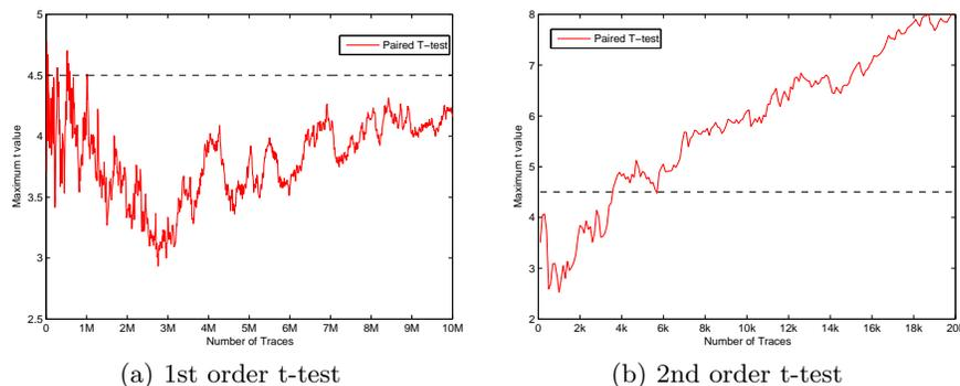
**Fig. 6.** Leakage detection results for the two-share implementation of Present for first order (left) and second order (right) leakage over the number of traces.
