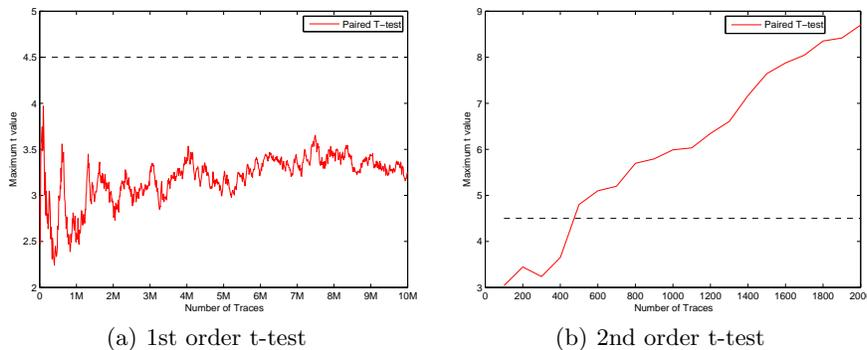
**Fig. 5.** Leakage detection results for the two-share implementation of Simon for first order (left) and second order (right) leakage over the number of traces. Note that the dimensions change for both axes.
