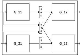
**Fig. 2.** Hardware architectures of 2-share G module
