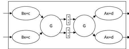
**Fig. 3.** Hardware architectures of 2-share S-box module
