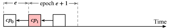
(a) Step 1: Byzantine validators delay checkpoint cp_1 for one slot. All Byzantine attestors in epoch e + 1 withhold their attestations.
