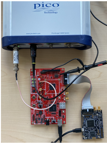
Fig. 7: Experimental setup for capturing power traces.
