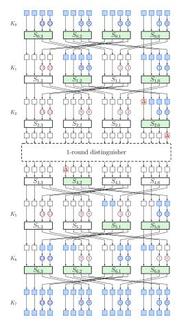
**Fig. 2.** Our toy cipher and a differential attack against it. S-boxes in green are active. Bits with a difference  $\Delta$  are active bits, while bits in blue are bits with an unknown difference (0 or 1). Bits in a circle correspond to key bits. Those in blue, are the ones that need to be guessed during the attack.
