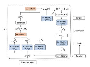
Figure 3. Overview of secure transformer inference in BERT.
