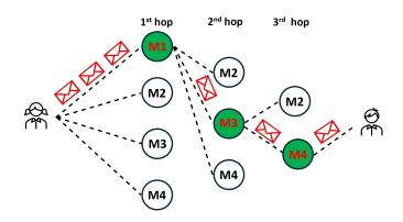
Fig. 2: Example of mixnode selection in a Free Routes mixnet.
