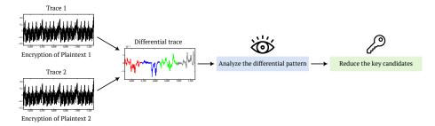
Figure 4: Illustration of one iteration of SCADPA methodology developed in [BJB18]. The attacker can repeat this process until the master key is found or until it can be searched with a reasonable time complexity.
