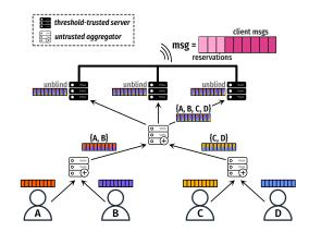
(b) An anonymous broadcast round in ZIPNet. Ciphertexts are XORed through multiple aggregation layers, until the root aggregator broadcasts the aggregate and user list to all servers. The servers then unblind and combine the aggregates into the final broadcast message.
