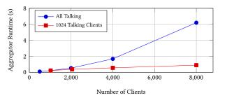
(a) Aggregator Computational Runtime as Number of Talking Clients Increase (and Broadcast Channel Increases) or as Cover Traffic Increases. Messages size is 160B.
