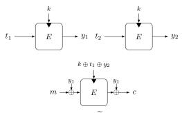
Figure 4: The first TBC construction  $\tilde{G}^1$  based on three block cipher calls.
