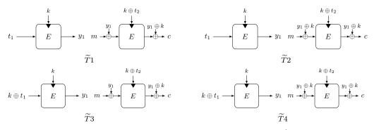
Figure 1: The four TBCs with two positions for tweak. Wang et al. [WGZ<sup>+</sup>16] showed that these TBCs has *n*-bit security when  $t_1 = t_2 = t$ . Here we consider the case when both  $t_1$  and  $t_2$  can be arbitrarily chosen by the adversary.
