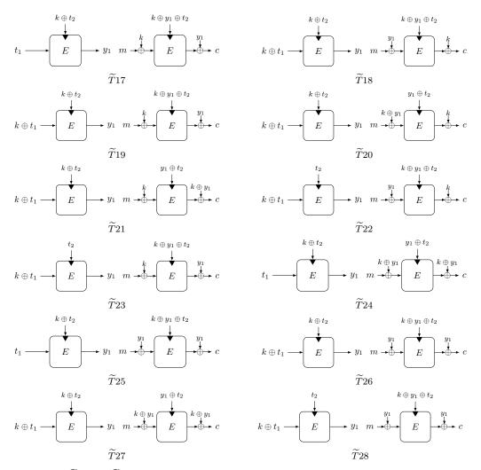
Figure 7:  $\widetilde{T}17$  to  $\widetilde{T}28$  of the 24 TBCs with constraints  $(\Delta_1, \Delta_2, \Delta_3) = (t_1, t_2, t_2)$  and  $(b_{12}, a_{12}, a_{22}) = (1, 1, 1)$  for 2*n*-bit tweak  $t_1$  and  $t_2$ .
