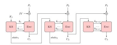
Fig. 1. The First Method for Implementing RK-CBC when m = 3.
