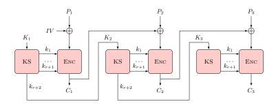
Fig. 2. The Second Method of Implementing RK-CBC when m = 3 and n = k.
