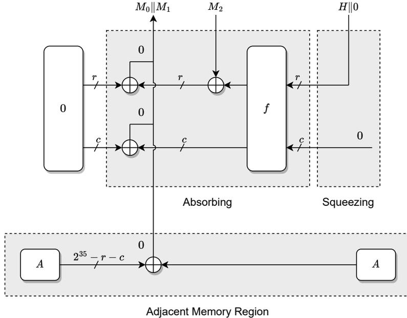
**Fig. 4.** SHA-3 preimage of any  $H$  for a vulnerable implementation. We use two calls to `Keccak_HashUpdate()` to process a message  $M_0||M_1$  that is again 4 GiB in length. However, we now use the fact that  $f$  is invertible to determine the correct value of  $M_0||M_1$ , noting that we can use the vulnerability to overwrite all  $r + c$  bits of the sponge state.
