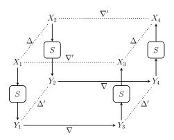
Figure 2: An S-box in the boomerang switch.
