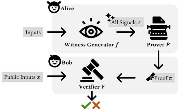
Figure 2: Usage of zero-knowledge proof: Alice generates a proof using witness generator and prover, and Bob verifies the proof using public inputs.
