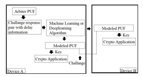
Fig. 1. Key exchange using PUF
