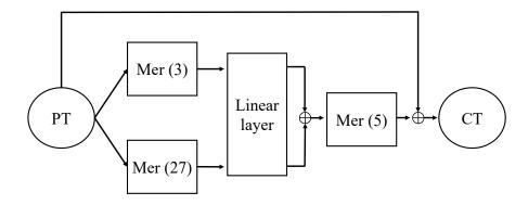
Fig. 1: AIM-I cryptographic process.
