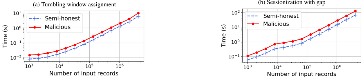
Figure 6: Scalability of the secure window assignment primitives, as the time series size increases from 2^{10} to 2^{22} (LAN).
