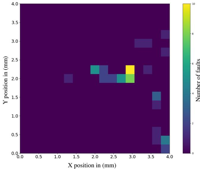
Figure 15: Successful EMFI effect on the glitchable application of ESP32-V3
