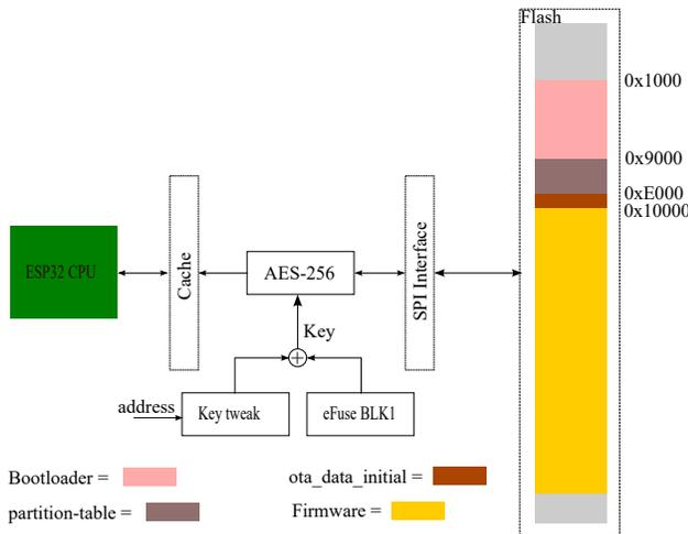
Figure 7: Flash encryption of ESP32
