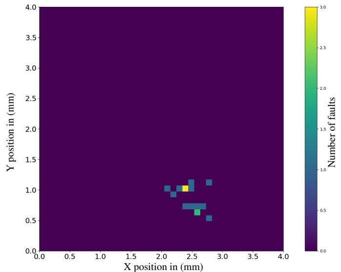
Figure 14: Successful fault map on ESP32-V1
