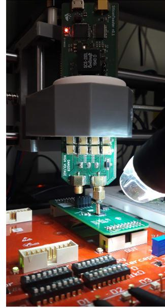
Figure 10: EM probe on ESP32
