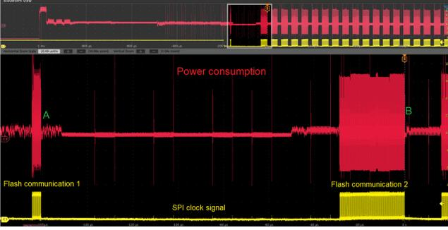
Figure 24: Power up during flash encryption
