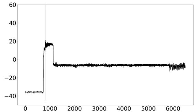
Figure 13: Power consumption in case of a successful fault of ESP32-V1
