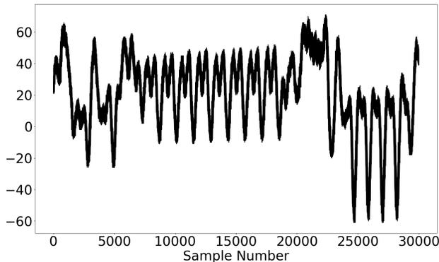
Figure 20: Power traces during the execution of List. 6 (50 traces without alignment)
