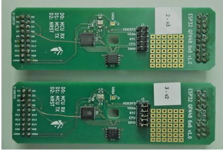
Figure 8: Fabricated PCB for ESP32
