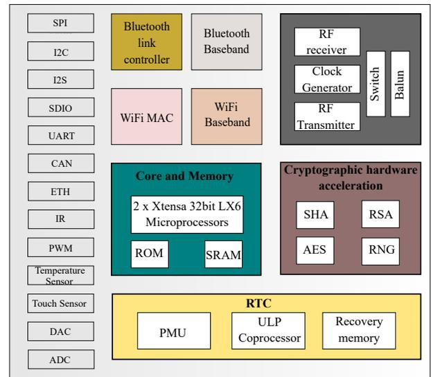
Figure 1: ESP32 architecture [11]
