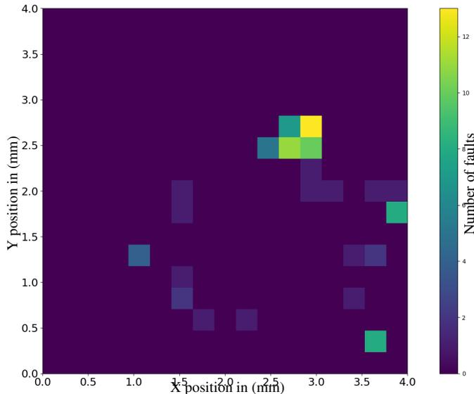
Figure 11: Successful fault map of the glitchable application
