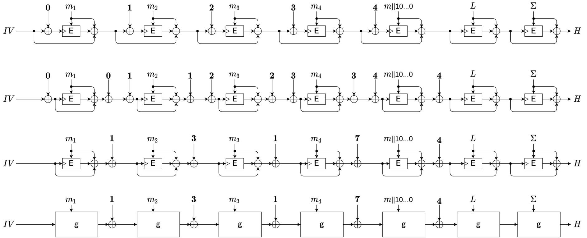
Figure 4: The equivalent representation of Streebog.
