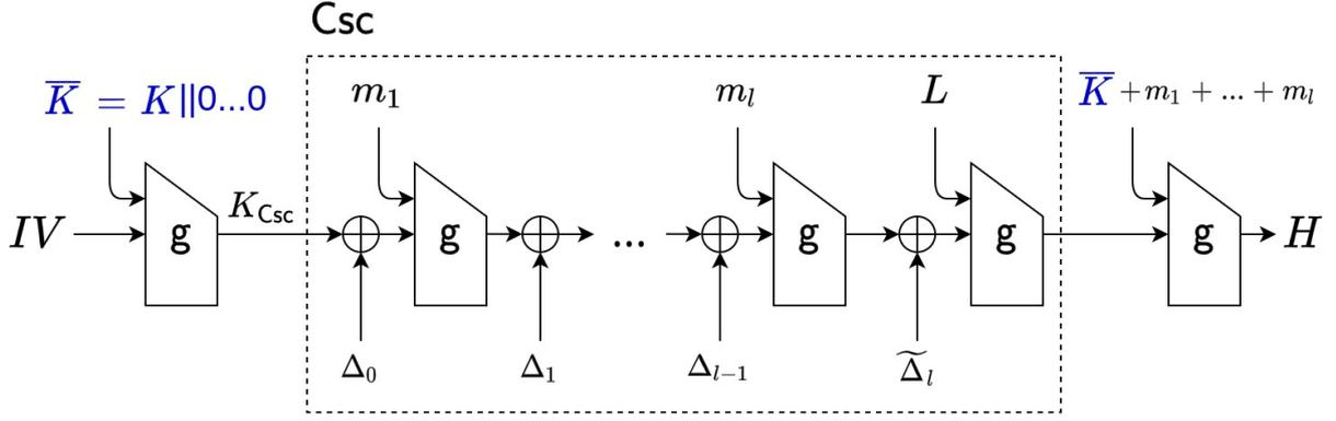
Figure 2: Streebog-K with the equivalent representation [22].
