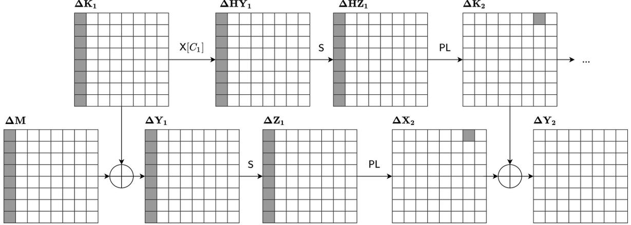
Figure 7: Online stage. Truncated related-key differential trail. The first round.  $\Delta M[\cdot, 0] \neq 0$ .
