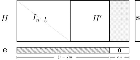
Fig. 4: Parity-check matrix in systematic form where  $\alpha n$  zero positions of  $\mathbf{e}$  are guessed. Striped region of  $\mathbf{e}$  indicates parts containing weight, crosshatched columns of  $H'$  do not affect  $\mathbf{s}$ . Framed parts are used as input to the quantum algorithm.
