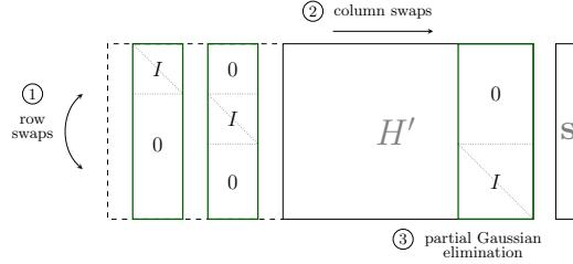
Fig. 3: Procedure to perform quantum version of Prange without first  $n - k$  columns as input. Colored framed parts indicate columns belonging to the current selected subset.
