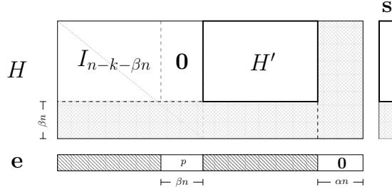
Fig. 8: Input matrix in systematic form where  $\beta n$  parity-check equations are omitted and  $\alpha n$  zeros of  $\mathbf{e}$  are known. The vector  $\mathbf{e}$  is assumed to contain weight  $p$  on  $\beta n$  coordinates. Framed parts are used as input to the quantum algorithm.
