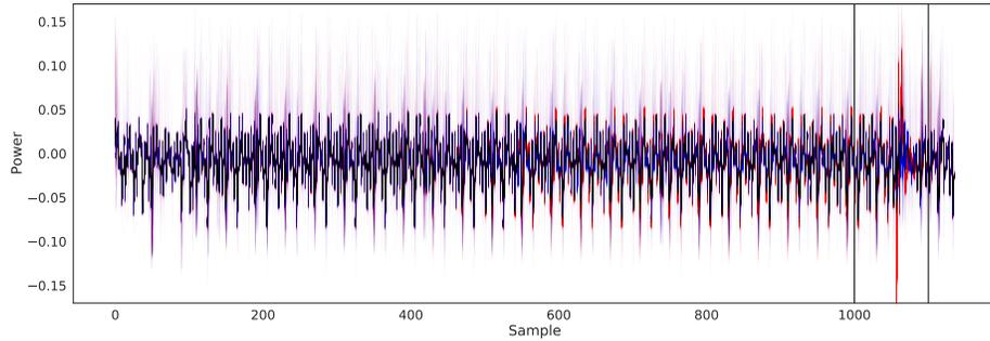
Fig. 4: 1,000 power traces of the FrodoKEM Gaussian sampler, modified to act as a two-sided sampler. Runs resulting in a negative sample are drawn in red, others in blue. The section marked by vertical lines shows the section used for training the classifier.
