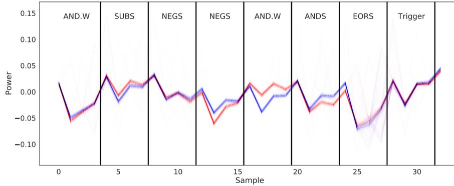
Fig. 3: GALACTICS Sign-Flip power trace annotated with the corresponding assembly instructions in the execute stage of the pipeline. Traces shown in red and blue had negative and positive return value, respectively.
