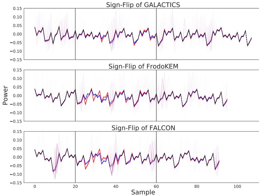
Fig. 2: 1,000 power traces of Sign-Flip implementations. Red and blue lines indicate negative and positive output, respectively. The section between the vertical black lines is used for training the neural network.
