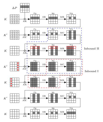
Fig. 16: Semi-free-start collision attack on 7-round Saturnin
