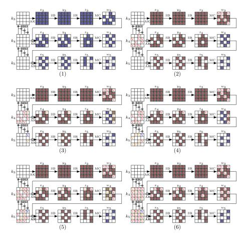
Fig. 9: Steps to recover  $k_5$ . The bytes marked by 'D' mean that the differences are known. The bytes marked by 'V' mean that the values are known. In subfigures, the bytes marked by 'V' are deduced from those marked by 'V'.
