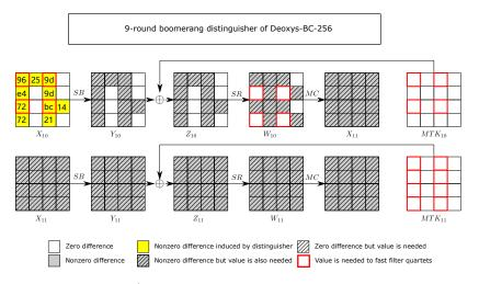
Figure 8: Rectangle/Boomerang attack on 11-round reduced Deoxys-BC-256
