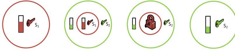
Fig. 4. Bootstrapping: Starting with a noisy ciphertext under secret key S_1 , represented by a red circle, bootstrapping will add another layer of encryption by encrypting the ciphertext under key S_2 with less noise. Next, the inner layer of encryption is stripped away by executing the decryption function homomorphically. The result is a ciphertext under key S_2 encrypting the same message with reduced noise.
