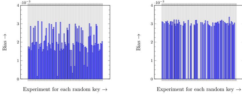
Fig. 4: Comparison of the biases for the case when Hamming weight of  $\Delta_m$  is 12 (left) vs 10 (right) after the first round. The experiment is done for 100 random keys  $k_i$  ( $i = 1, 2, \dots, 100$ ). Along  $x$ -axis, the  $i$ -th vertical line represents the bias corresponding to  $k_i$ . For each random key the probability is calculated over  $2^{28}$  random IVs.
