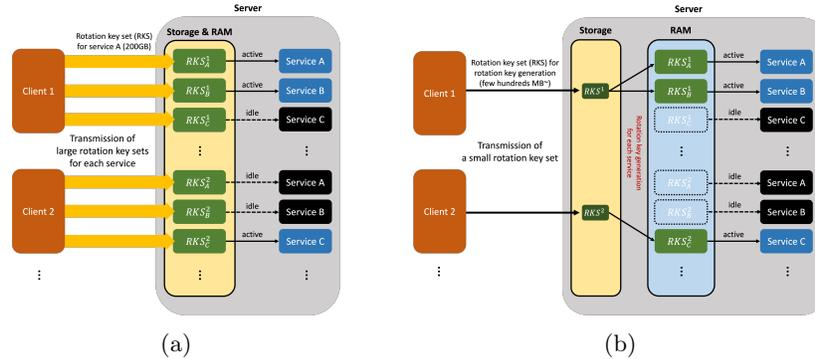
Fig. 1: Comparison of conventional rotation key system and hierarchical rotation key system for HE-based services in the client-server model (a) Conventional rotation key system (b) The proposed hierarchical rotation key system.
