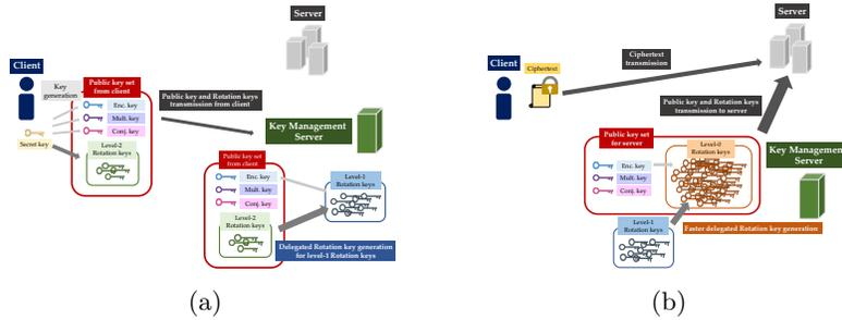
Fig. 2: Efficient rotation key management in three-level hierarchical rotation key generation. (a) Public key and level-2 rotation key transmission from the client and preparation for faster level-0 rotation key generation by generating level-1 rotation keys in advance. (b) Faster rotation key generation from public key and level-1 rotation keys.
