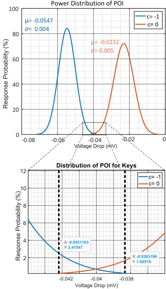
Fig. 5. The distribution of power measurements at the POI for the two different assignments (-1 vs. 0) during the targeted instruction in NTRU-HPS. These two power distributions intersect with each other and the intersection reduces the success rate.
