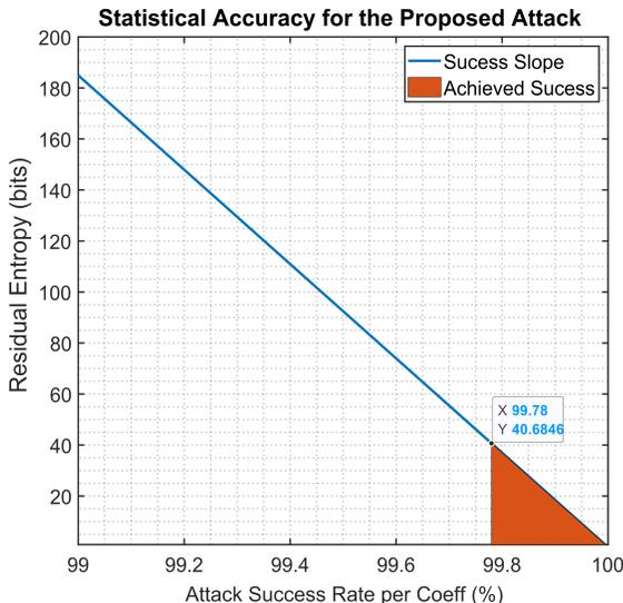
Fig. 7. The success rate of our proposed attack vs. the residual entropy of the session/secret keys in NTRU-HPS. Our per-coefficient success rate of 99.78% reduces the search space of keys to about  $2^{41}$ .
