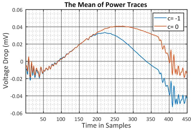
Fig. 2. The mean of sub-traces for different comparison results. There is a significant power consumption difference between these comparison results.
