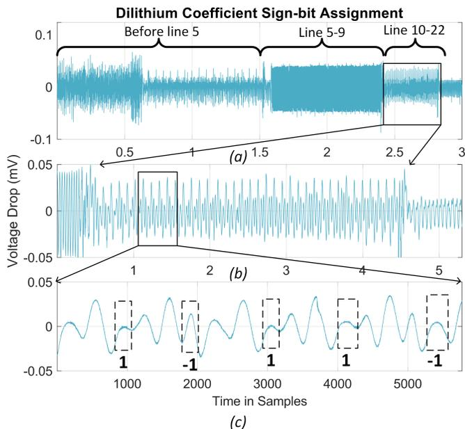
Fig. 3. (a) The full power trace, (b) the sub-trace showing the full for-loop, (c) the sub-trace for the 5 iterations of this for-loop. The regions of interests are detectable from the full power measurement and the coefficient assignments can be identified.
