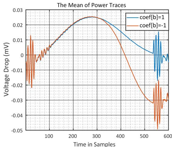
Fig. 4. The mean of sub-traces for different coefficient assignments. There is a significant power consumption difference between these assignments.
