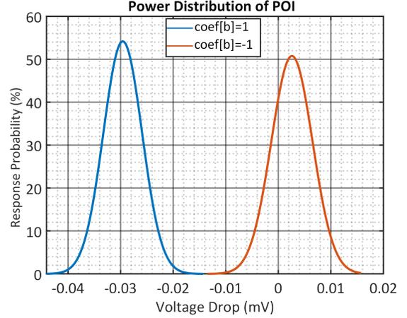
Fig. 6. The distribution of power measurements at the POI for the two different assignments (-1 vs. 1) during the targeted instruction in CRYSTALS-DILITHIUM. Although the two power distributions theoretically intersect with each other, the intersection cannot be seen visually.
