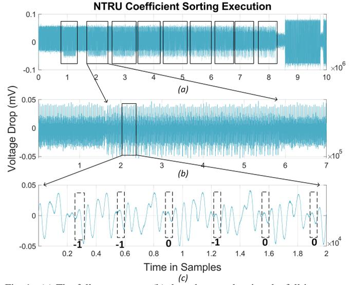
Fig. 1. (a) The full power trace, (b) the sub-trace showing the full innermost loop, (c) the sub-trace for the 6 iterations of the innermost loop. The regions of interests are detectable from the full power measurement and the comparison results can be identified.
