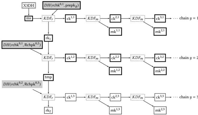
**Figure 2: The key schedule of Signal where the DH values are marked with grey boxes. Each stage  $(x, y)$  has its  $x$ -coordinate corresponding to a message (horizontal moves) inside a chain (vertical moves) for  $y$ -coordinate. The compromise (in double edge) during  $A$  setup is affecting the keys (in thick edge) of the two first chains.**
