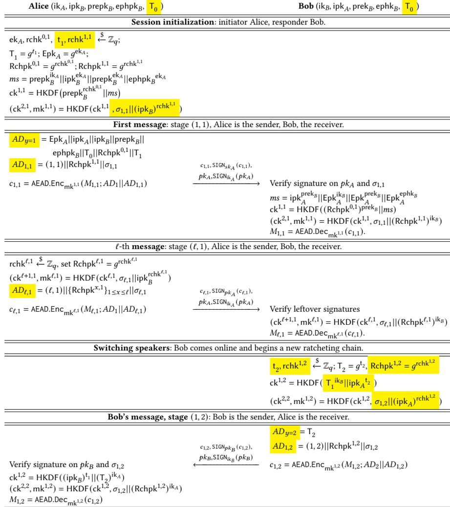
**Figure 3: MARSHAL protocol execution between Alice and Bob for the first few stages. The yellow boxes indicate modifications with respect to Signal protocol [8]. The transmitted data is also different and not in yellow for more clarity.**
