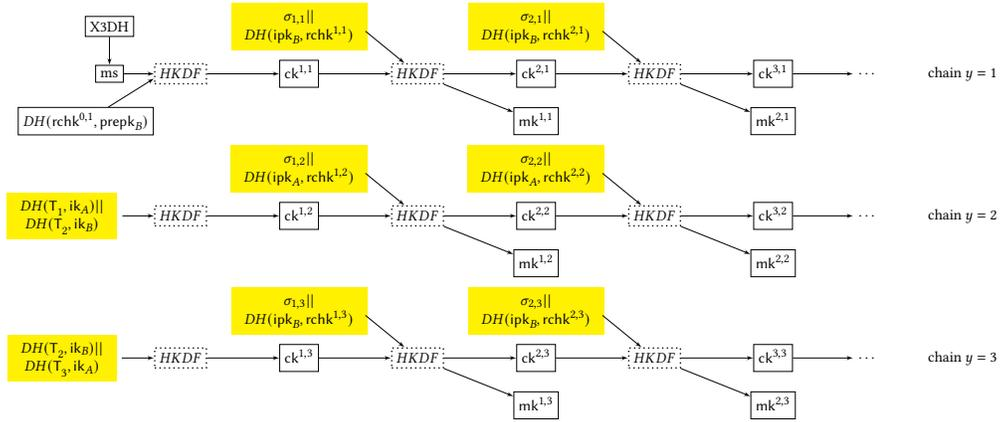
**Figure 4: MARSHAL key schedule diagram, where  $\sigma_{x,y} = \text{SIGN}_{sk_A}(T_{y-1} || \text{Rchpk}^{x,y})$  for  $y$  odd and  $\sigma_{x,y} = \text{SIGN}_{sk_B}(T_{y-1} || \text{Rchpk}^{x,y})$  for  $y$  even. The yellow boxes indicate modifications with respect to Signal protocol [8].**
