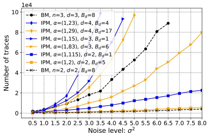
Figure 13. Attack-based evaluation of IPM with  $n = 2$  shares with y-axis in normal scale. Note that we take two codes in each group with different  $d_{\mathcal{D}}^{\perp}$  and/or  $B_{d_{\mathcal{D}}^{\perp}}$ .
