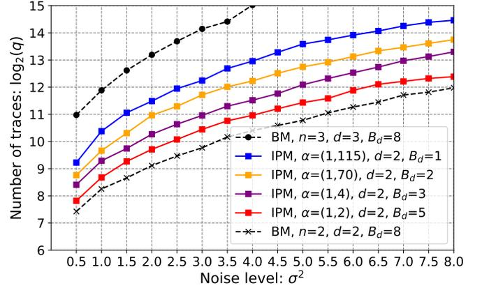
Figure 5. Illustrating the impact of  $B_{d_{\mathcal{D}}^{\perp}}$  given the same  $d_{\mathcal{D}}^{\perp}$  in 2-share IPM. Note that 2-share IPM instances have different kissing number  $B_{d_{\mathcal{D}}^{\perp}}$ .
