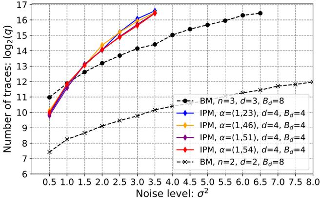
Figure 4. Comparison of four instances of optimal codes for 2-share IPM, according to the best coding-theoretic properties given by  $d_{\mathcal{D}}^{\perp} = 4$  and  $B_{d_{\mathcal{D}}^{\perp}} = 4$ . Note that the number of traces is shown only in  $\log_2$  scale for the sake of brevity.
