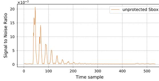
Fig. 2. SNR for the *unprotected AES Sbox*.
