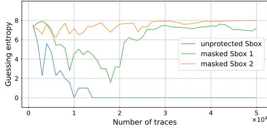
Fig. 6. The *guessing entropy* of the 8-bit secret key, after correlation power analysis on an *unprotected Sbox* (blue line) and two protected AES Sbox implementations: *masked Sbox 1* (green) and *masked Sbox 2* (orange).
