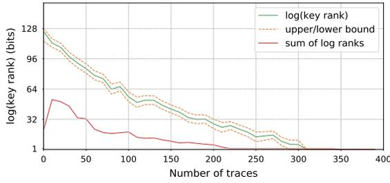
Fig. 8. Unprotected AES Sbox, simulated leakage ( $\sigma = 1$ ).
