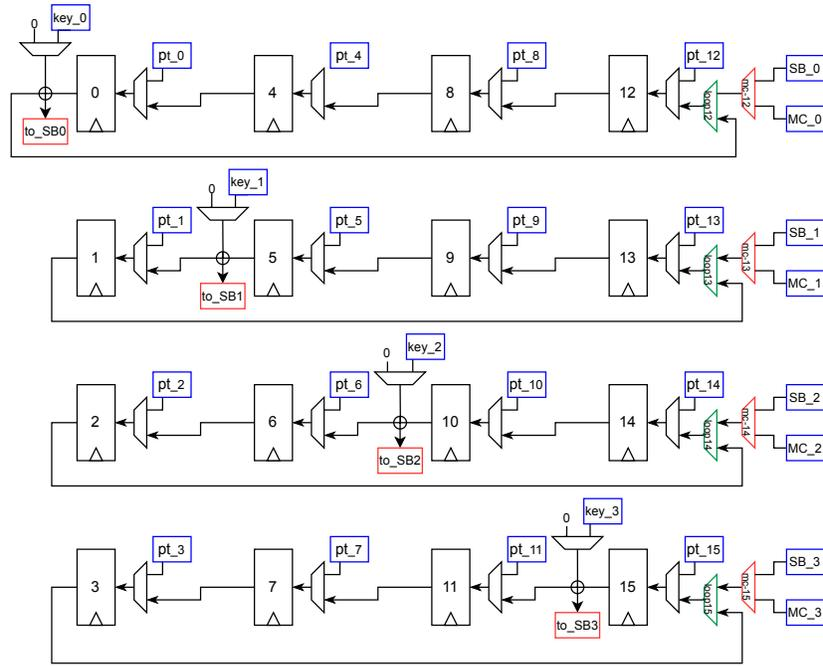
**Fig. 7.** 32-bit implementation: architecture of the state holder.
