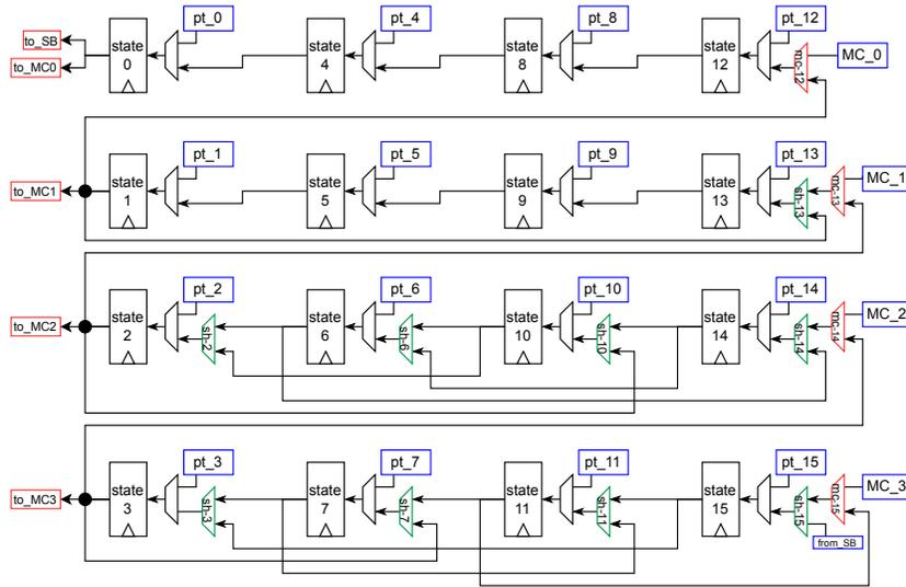
Fig. 4. 8-bit implementation: architecture of the state holder.
