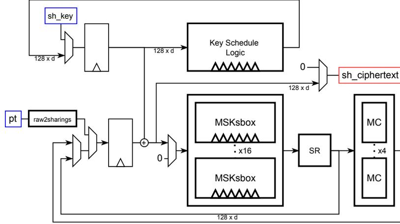
Fig. 9. Global Architecture of the 128-bit serial implementation
