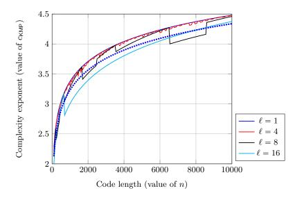
Fig. 4: Complexity exponents for the KMP algorithm, as a function of n, for the case of  $\ell = 1$ . Continuous lines report the values of  $c_{\text{KMP}}$  arising from Proposition 6, while dotted lines report the values of  $c_{\text{KMP}}^*$ .
