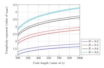
Fig. 3: Complexity exponents for the KMP algorithm, as a function of n, for the case of  $\ell = 1$  and several code rates (indicated by R). Continuous lines report the values of  $c_{\text{KMP}}$  arising from Proposition 6, while dotted lines report the values of  $c_{\text{KMP}}^*$ .
