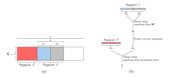
Fig. 6: Graphical representation of the algorithm in [25]. Figure (a) describes how the coordinates of the solution  $\tilde{\mathbf{V}}$  are partitioned; figure (b) shows lists operations. The use of colors in both figures is coherent, for instance: list  $\mathcal{K}_2$  in figure (b) contains candidates for the submatrix of  $\tilde{\mathbf{V}}$  colored in grey.
