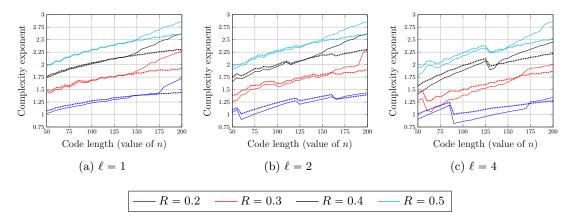
Fig. 8: Complexity exponents for our algorithm and KMP, for  $\ell = 1$  and several code rates (indicated by R). Continuous lines are referred to our algorithm, dotted lines to the KMP algorithm.
