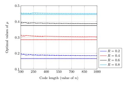
Fig. 2: Values of  $\mu$  that optimize the KMP algorithm, for  $\ell = 1$  and several code rates (indicated by R). The continuous line has been obtained by selecting, among all possible choices for  $(u_1, u_2)$ , the ones yielding the smallest value for  $T_{\mathsf{KMP}}(u_1, u_2)$ . Dashed lines report the optimal values of  $\mu$  which we have found by numerically solving (11). Dotted lines correspond to  $\mu^* = \frac{R}{1+R}$ .
