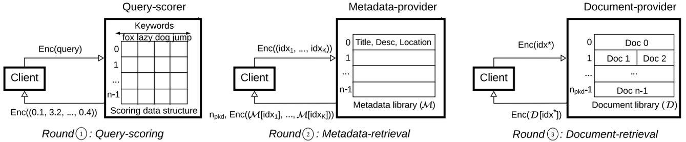
Figure 1. An overview of Coeus’s three-round protocol: query-scoring, metadata-retrieval, and document-retrieval.
