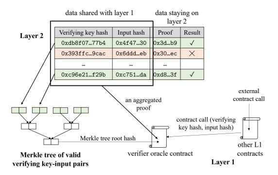
Figure 1: System architecture of zk-BatchVerify.
