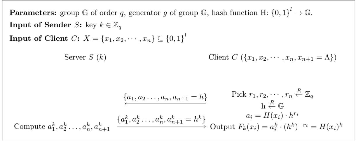
Figure 6: Our improved Hashed DH multi-point rOPRF using Multiplicative Blinding
