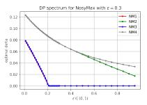
(c) Estimated  $(\varepsilon, \delta)$  spectrum of four variants of Noisy max. NM1 and NM3 [8, Alg.5, 6] satisfy  $(\varepsilon = 0.3, \delta = 0)$ -DP while NM2 and NM4 [8, Alg.7, 8] do not.
