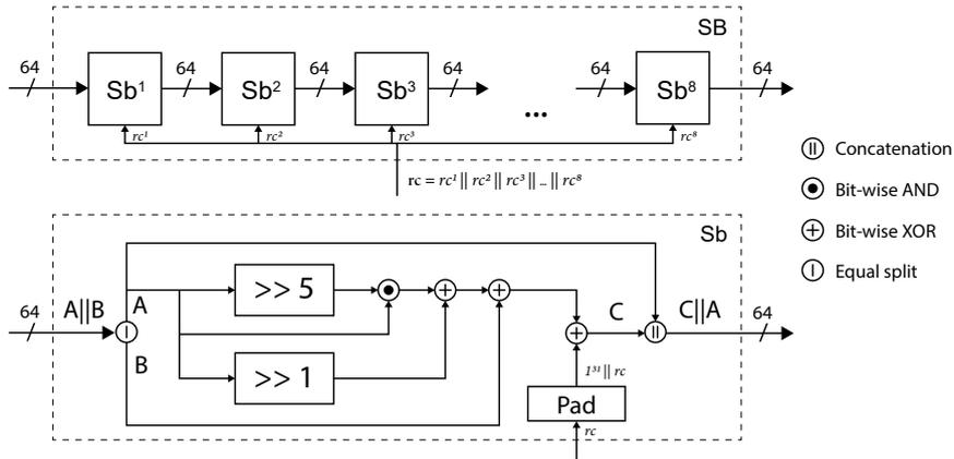
Fig. 2: Simeck box (SB) and Sub-Simeck box (Sb)
