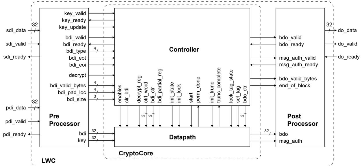
Fig. 5: Top level block diagram of LWC core
