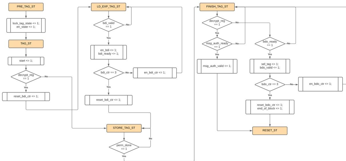
Fig. 9: Tag generation and Controller reaching reset state
