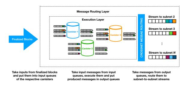
Figure 3: Message routing and execution layers
