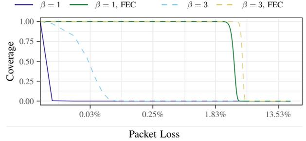
Figure 2: Reliability of UDP-based block propagation over unreliable channels (block size of 1 MB,  $L = 160$ , and FEC overhead factor  $f = 0.15$ ).
