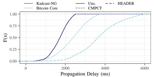
Figure 8: Block propagation delays for *kadcast-ng* and Bitcoin Core in a testbed of 1,000 nodes.
