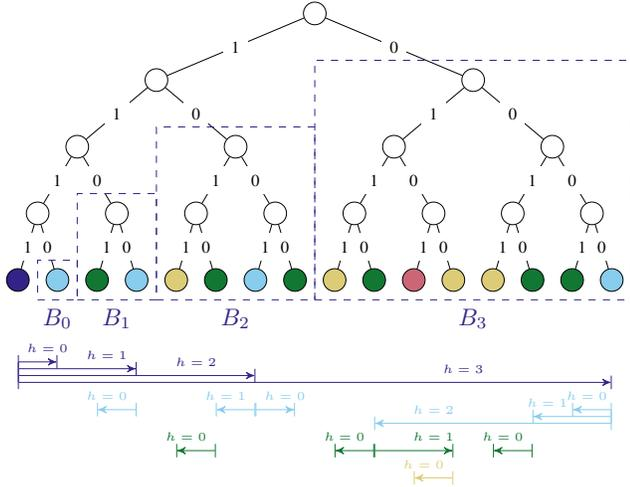
Figure 1: Example broadcast initiated by node 1111 ( $\beta = 1$ ). Colors indicate node distances in the spanning tree, relative to the initiator.
