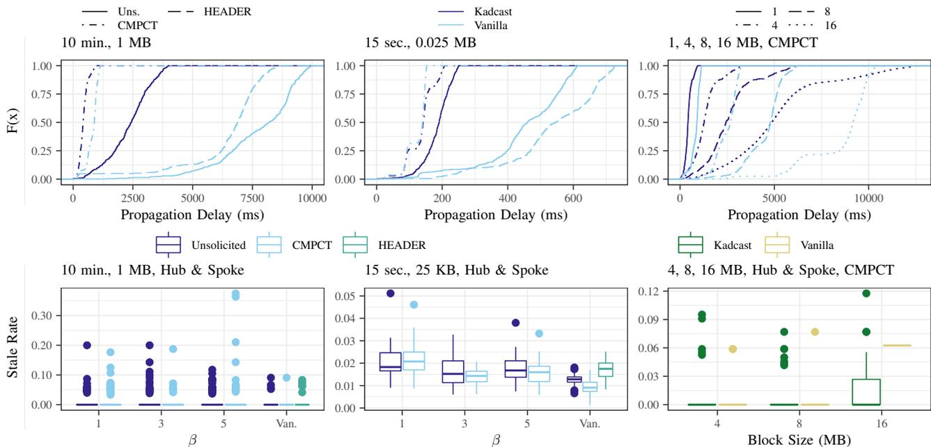
Figure 4: Block propagation delay and resulting stale rates for Bitcoin-like and Ethereum-like parametrizations, as well as for simulation scenarios with higher block size limits.
