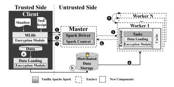
Fig. 2: SOTERIA architecture and operations flow.
