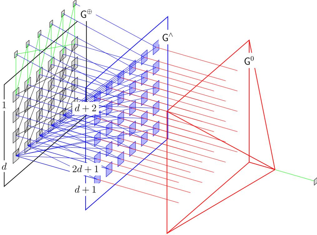
Figure 1: Schematic diagram for the candidate circuit of width 5 and depth 4. The input and output wires are coloured green. The layer number is indicated on the left. The first two blocks are the XOR and AND layers respectively; the final pyramid denotes the binary tree.
