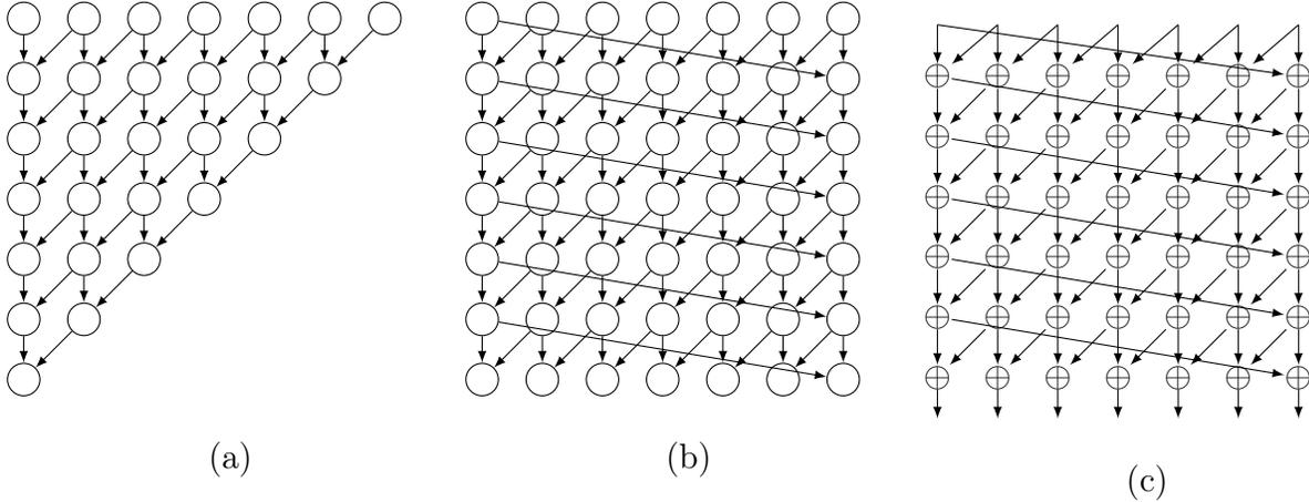
Figure 2: The graphs and the circuit for parameter  $d = 6$ : (a) A pyramid graph of depth  $d$ , (b) Extending the pyramid graph to get a tower graph  $G_d^\oplus$  of depth  $d$  and (c) Circuit  $G_d^\oplus$  obtained replacing the vertices in  $G_d^\oplus$  with XOR gates.
