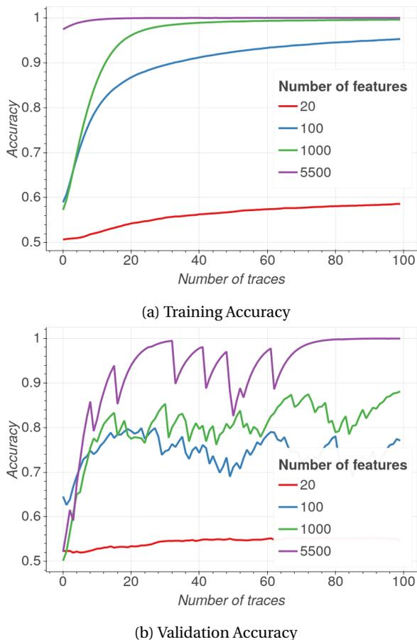
Figure 8: Accuracy of the CNN method over 100 epochs on the protected implementation dataset.
