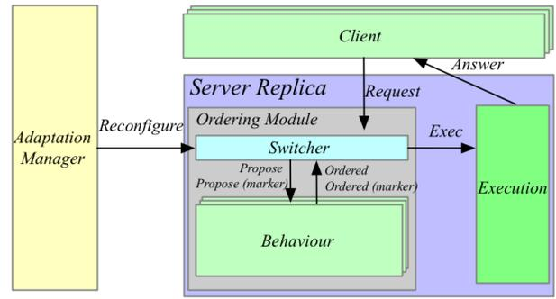
Fig. 50. System architecture of dynamic BFT adaption [265].
