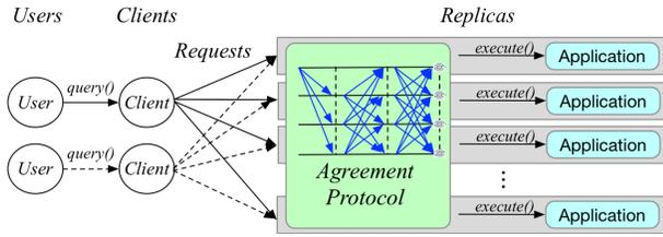
Fig. 2. Abstract of BFT replication system. Users send requests to replicas via client interfaces (with well-defined client library). Replicas together run an agreement protocol to obtain an order on clients’ requests, and then each replica executes them in its stateful application [6].
