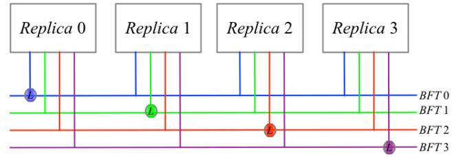
Fig. 41. In the fault-free case, each replica leads one of the BFT agreement protocol instances [236].
