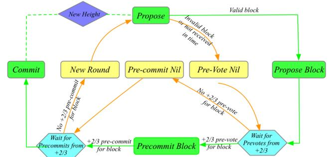
Fig. 43. After the proposal step, validators only make progress after hearing from two-thirds or more ( $+2/3$ ) of other validators. The dotted arrow extends the consensus into atomic broadcast by moving to the next height [237].
