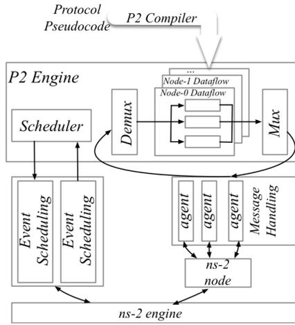
Fig. 24. The BFTSim software architecture [63].
