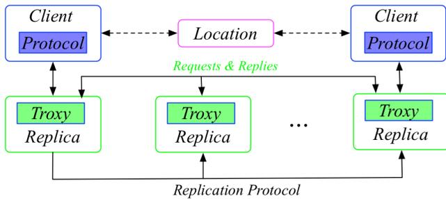
Fig. 47. Architecture of a Troxy-backed BFT system [254].
