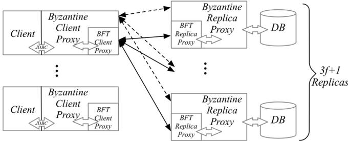
Fig. 25. Byzantium system architecture [193].
