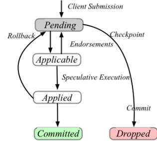
Fig. 8. Transaction state diagram, as viewed by a node. From the Pending state, a transaction evolves either to Dropped or Committed given received messages. Dropped and Committed are eventually consistent across all nodes. However, Pending, Applicable, and Applied are intermediate states local to each node which might not be consistent [104].
