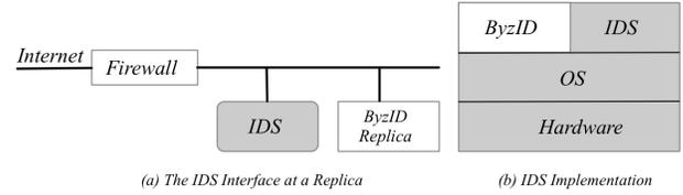
Fig. 35. The IDS/ByzID architecture. Gray components is trusted [222].
