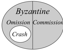
Fig. 26. Failure hierarchy. Byzantine failures include omission failures and commission failures. Crash failures are a subset of omission failures [198].
