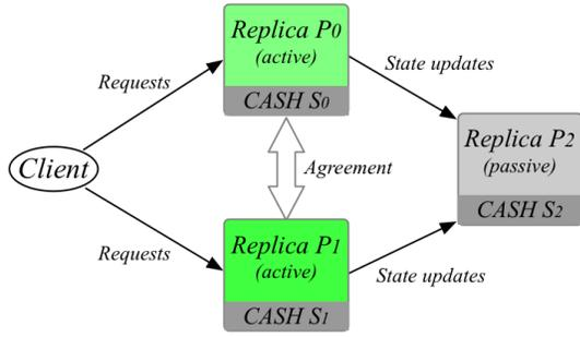
Fig. 12. CheapBFT architecture with two active replicas and a passive replica ( $f = 1$ ) for normal-case operation [161].
