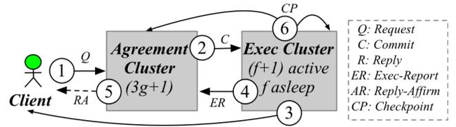
Fig. 28. The normal agreement and execution protocol in ZZ proceed through steps 1-5. Step 5 is needed only after a fault. Checkpoints (step 6) are created on a periodic basis [215].
