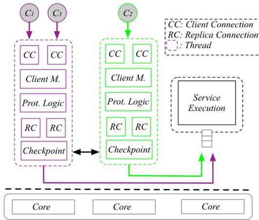
Fig. 39. Replica with self-contained pillars of a Consensus-oriented Parallelization (COP) [229].
