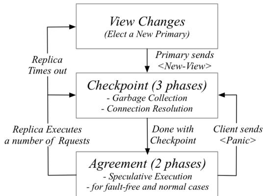
Fig. 38. Layered structure of hBFT [228].
