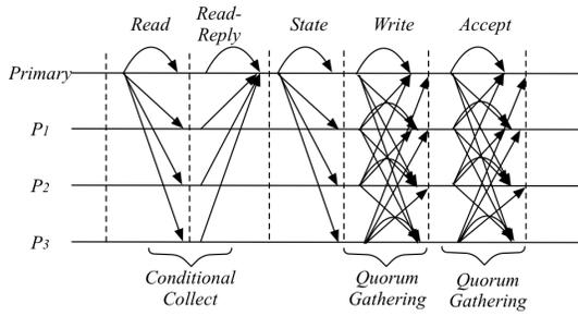
Fig. 40. VFT-SMaRt communication pattern [234].
