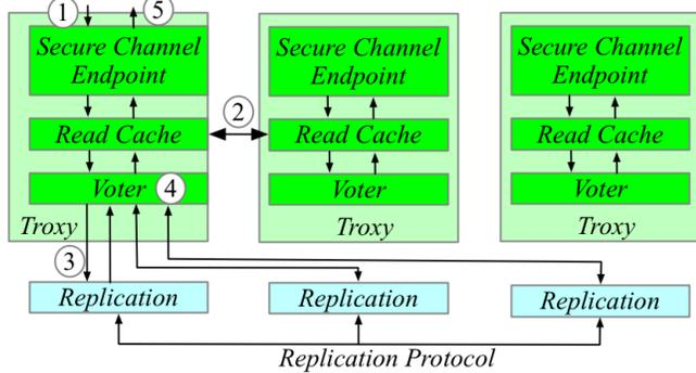
Fig. 48. Overview of Troxy components and their interactions [254].
