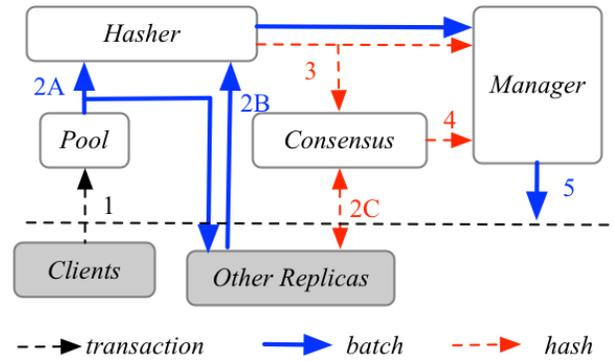
Fig. 54. Architecture of DISPEL. Transactions are collected in the pool and batched (1). Replicas exchange batches (2A, 2B), store and associate them with their hash digest in the manager (3). Replicas execute consensus protocol over hashes (2C, 3) and transmit the decisions to the manager (4). The manager transmits the batches associated with the decided hashes to the application (5) [280].
