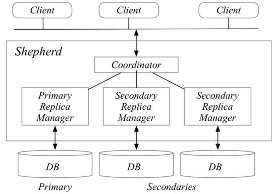
Fig. 23. HRDB system architecture [184].
