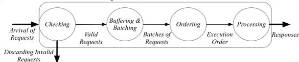
Fig. 37. Pipeline: an abstract for request processing in aPBFT [227].
