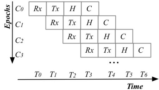
Fig. 55. Principle of a consensus pipeline. A pipeline epoch consists of four phases: network reception (Rx), network transmission (Tx), CPU intensive hash (H) and latency bound consensus (C). As soon as an epoch finishes its first phase (Rx), the replica spawns a new epoch. When the replica executes four epochs concurrently, it leverages all its resources [280].
