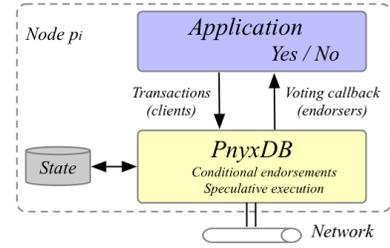
Fig. 7. Overview of PnyxDB. The application submits transactions to be executed on shared state and polls the application back for transaction approval before creating conditional endorsements [104].
