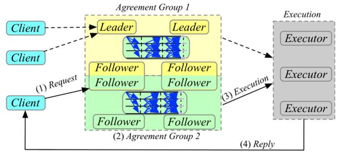
Fig. 14. An overview of the OMADA architecture relying on multiple, possibly overlapping, agreement groups. To invoke an operation at the application, a client (1) sends a request to one of the agreement groups, which then (2) orders the request using PBFT and (3) forwards it to a set of executors. Having processed the request, (4) the executors return their results to the client. [162].
