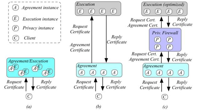
Fig. 20. High level architecture of (a) traditional Byzantine BFT SMR, (b) separate BFT agreement and execution, and (c) optimization-enabled by separation of agreement and execution [176].
