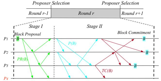
Fig. 10. Overview of a Gosig round without pipelining [127].
