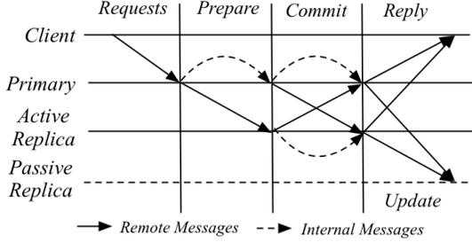
Fig. 13. CheapTiny protocol messages exchanged between a client, two active replicas, and a passive replica ( $f = 1$ ) [161].
