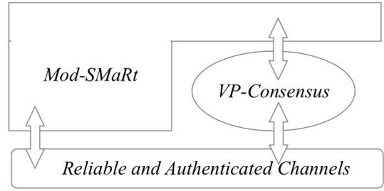
Fig. 29. Mod-SMaRt replica architecture. The reliable and authenticated channels layer guarantee the delivery of point-to-point messages, while the VP-Consensus module is used to establish agreement on messages to be delivered in a consensus instance [23].
