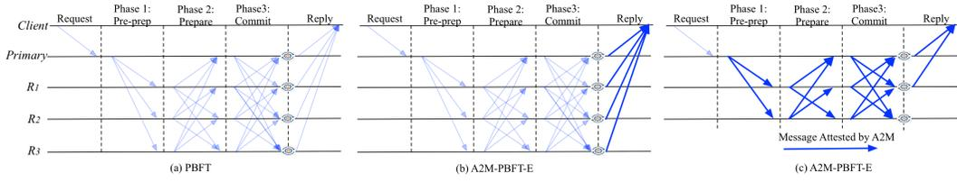
Fig. 11. Three-phase agreement protocol. Thicker lines denote messages that are attested by A2M [144].
