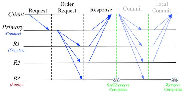
Fig. 17. The communication patterns of Zzyzyva and SACZyzyva with one faulty replica. Without faults or network delays, Zzyzyva and SACZyzyva have identical communication patterns, but if any replicas are faulty, Zzyzyva requires two extra rounds of communication [79].
