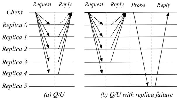
Fig. 4. Message patterns of Q/U. (a) Q/U common case operation, (b) Q/U with replica failure.
