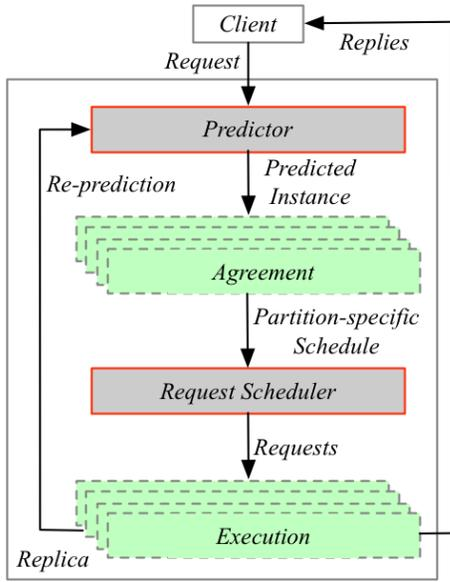
Fig. 42. System architecture of SAREK [236].
