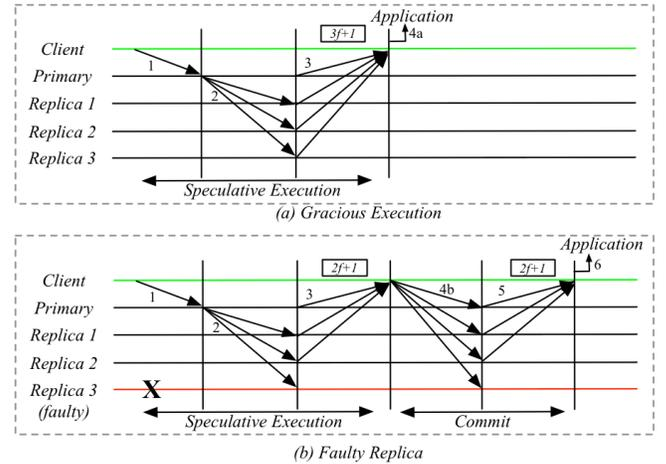
Fig. 5. Protocol communication patterns within a view for (a) gracious execution and (b) faulty replica cases. The numbers refer to the main steps of the protocol numbered in the text [59].
