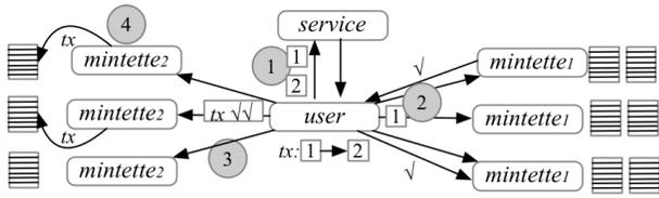
Fig. 44. The process of validating transactions; each mintette  $m_i$  is an owner of address  $i$ . In (1), a user learns the owners of each of the addresses in its transaction. In (2), the user collects approvals from a majority of the owners of the input addresses. In (3), the user sends both the transaction and these approvals to the owners of transaction identifier. In (4), some subset of these mintettes add the transactions to their blocks [239].
