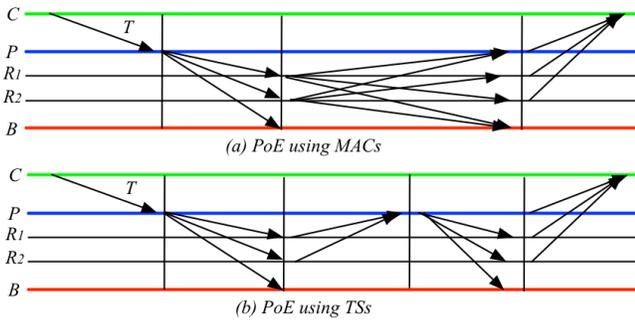
Fig. 56. Normal-case algorithm of PoE: Client  $c$  sends its request containing transaction  $T$  to the primary  $P$ , which proposes this request to all replicas. Although replica  $B$  is Byzantine, it fails to affect PoE [282].
