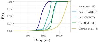
Fig. 6. Block propagation times as simulated by bns in comparison to realworld measurements and results by other blockchain simulators.
