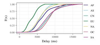
Fig. 8. Propagation delays in dependence of miner's geographic location.
