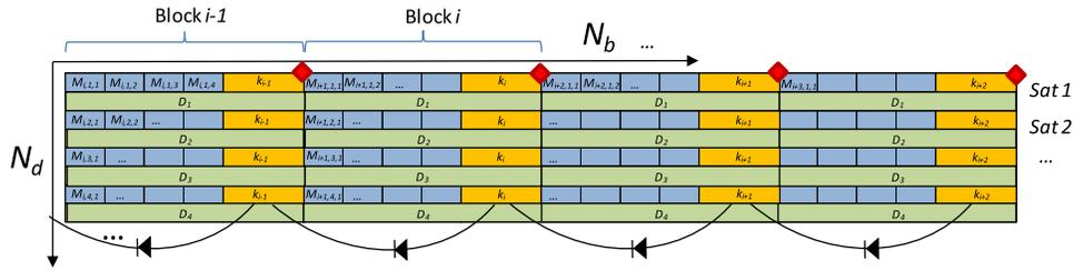
Fig. 1. GNSS-TESLA data structure for a MAC and key block from multiple satellites. Each satellite transmits its data ( $D$ ), several MACs ( $M$ ) and the key ( $k$ ).  $N_d$  is the number of datasets authenticated in each block and  $N_b$  the number of blocks within the attack period. Each diamond represents that the key has been fully received and verifications of MACs from the preceding block can commence.
