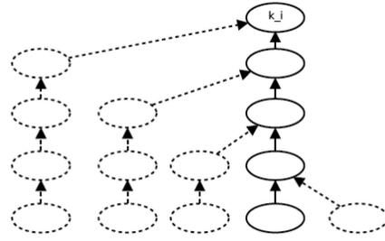
Fig. 3. Tree of chains ending in  $k_i$ . Keys along the original chain are connected via a solid line, while ineffective keys are drawn with a dotted line. An effective key (solid circle) has two incoming arrows: one from an effective key (solid circle), and one from an ineffective key (dotted circle) which was mapped at random according to (7); ineffective keys have only a single incoming arrow from a randomly mapped preimage according to (7).
