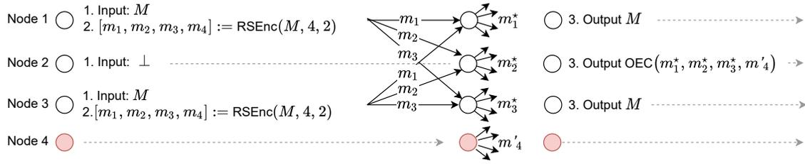
**Figure 2:** A example execution of our solution to ADD with 4 nodes  $\{1, 2, 3, 4\}$  among which node 4 is malicious and node 2 does not start with  $M$ . As described, after the dispersal phase, node 2 will receive  $2 = t + 1$  identical copies of  $m_2$  from node 1 and 4 and hence will set  $m_2$  as  $m_2^*$ . As a result, after the reconstruction phase, node 2 will receive 3 correct symbols of  $M'$  which is sufficient for reconstructing  $M$ .
