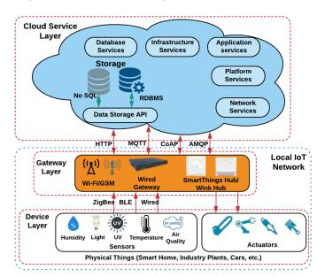
Fig. 2. An overview of a typical cloud-based IIoT infrastructure.
