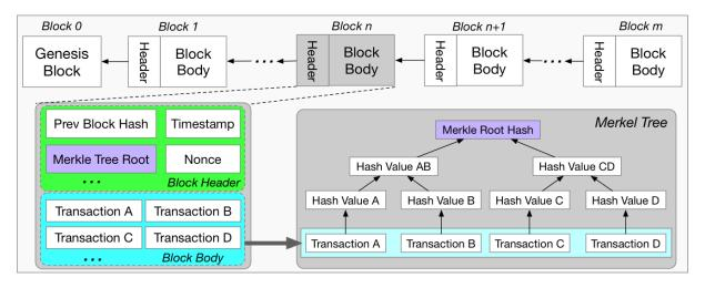
Fig. 3. Overview of blockchain. Blocks are linked in a inverse manner to its previous block, and each block contains a block header (e.g., metadata information) and a block body (e.g., transactions). The Markle tree root of transactions will be stored in block header.
