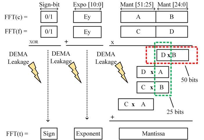
Fig. 2. The proposed attack on FALCON's floating-point multiplications. Targeting multiplications (shown in red dashed lines) creates false positives and targeting intermediate additions (shown in green dashed lines) eliminates them.
