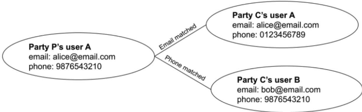
Figure 1: An example of many-to-many connections with multiple identifiers
