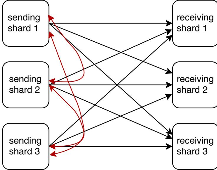
Figure 6: Cross Shard Shuffle with 3 shards
